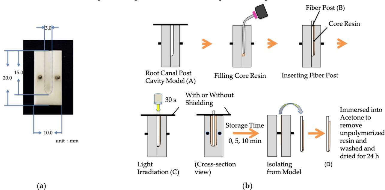
Figure 2. (a) The mold of the root canal cavity model. (b) Method of sample preparation.
