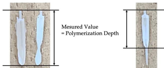
Figure 3. Polymerization Depth
