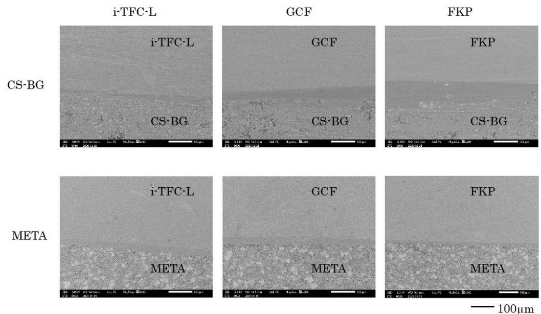
**Figure 5.** SEM micrographs of the surfaces of bonded interface between core resin and root canal sealer (200×). Adhesive surface is observed in CS-BG group and META group regardless of type of core resin.
