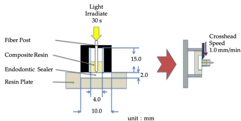
**Figure 4.** The schema of experiment sample.
